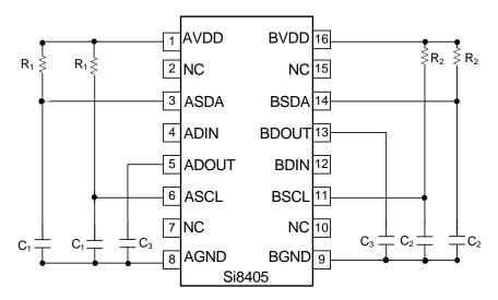
Figure 2. Simplified Timing Test Diagram
