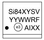
Figure 22. 8-Pin Narrow Body SOIC Top Marking
