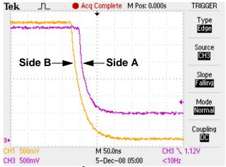
Figure 4. I<sup>2</sup>C Side B Pulling Down
