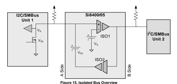
The "A side" output low  $(V_{OL})$  and input low  $(V_{IL})$  levels are designed such that the isolator  $V_{OL}$  is greater than the isolator  $V_{IL}$  to prevent the latch condition.
