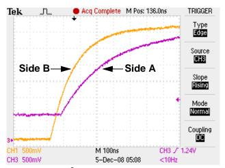
Figure 5. I<sup>2</sup>C Side B Pulling Up, Side A Following
