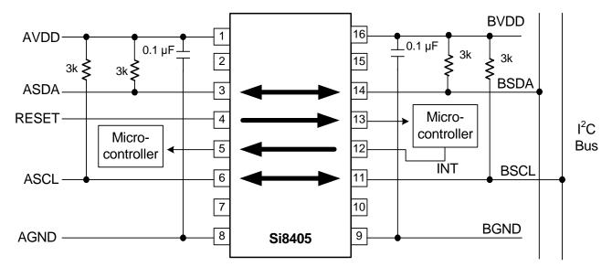
**Figure 16. Typical Application Diagram**
