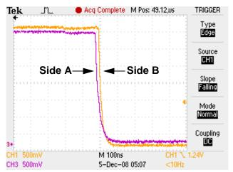
Figure 3. I<sup>2</sup>C Side A Pulling Down (1100  $\Omega$  Pull-Up)
