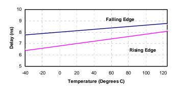
Figure 7. Non I<sup>2</sup>C Channel Propagation Delay vs. Temperature
