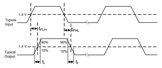
Figure 1. Propagation Delay Timing (Non-I<sup>2</sup>C Channels)
