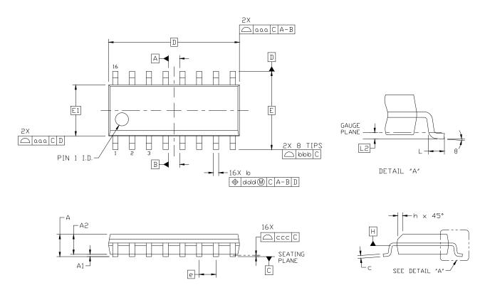
Figure 20. 16-pin Small Outline Integrated Circuit (SOIC) Package
