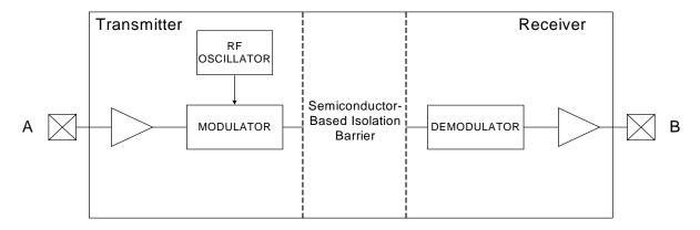
Figure 10. Simplified Channel Diagram
