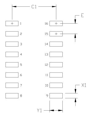
Figure 21. 16-Pin Narrow Body SOIC PCB Landing Pattern
