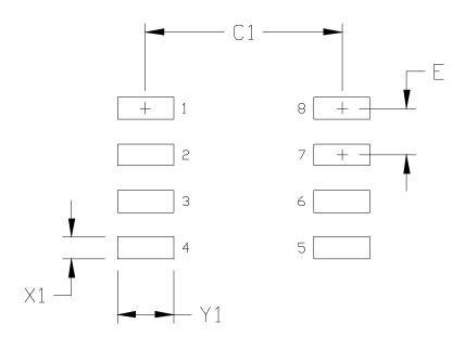
Figure 19. PCB Landing Pattern: 8-Pin Narrow Body SOIC
