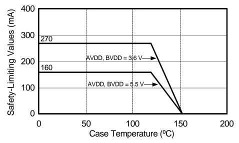
Figure 8. NB SOIC-8 Thermal Derating Curve, Dependence of Safety Limiting Values with Case Temperature per DIN EN 60747-5-2
