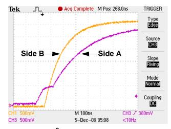
Figure 6. I<sup>2</sup>C Side A Pulling Up, Side B Following
